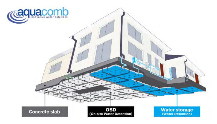
Aquacomb is an innovative water storage solution that collects and retains rainwater for your home. This unique water harvesting system comprises a series of interconnected water storage pods which are housed wholly within a concrete slab or under any hard covered surface. If you also require OSD (on-site water detention) the Aquacomb system is the perfect combination all-in-one system, which is totally out of sight.
